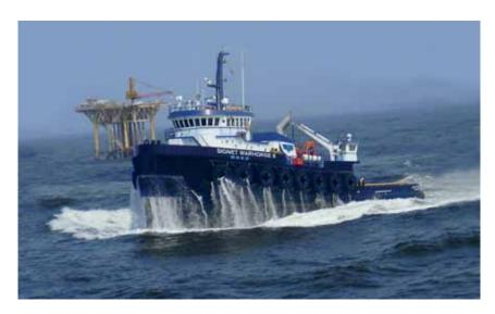
Demonstrating its strength, the SIGNET WARHORSE II, is the most powerful ABS classed ocean towing vessel in Signet Maritime's Offshore Towing Division. At 153.58 tonnes bollard pull, the SIGNET WARHORSE II will lead the fleet providing ocean towing of rigs, spars and other vessels.
